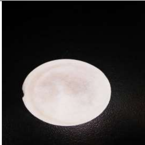
Figure 6: Filter paper after dried for one hour (TSS test)
