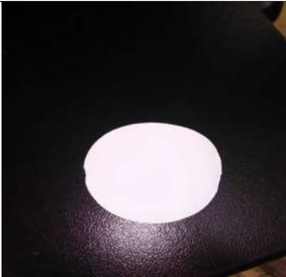
Figure 5: Filter paper before (TSS test)
